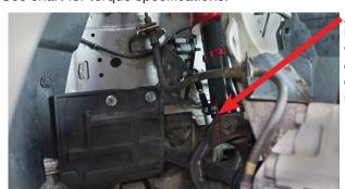
Align the lower bracket with the outside edge of the lower mount arm.
